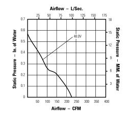
All operating specifications measured at nominal operating voltage, free air at sea level
